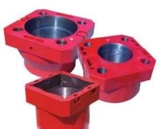
MKP Master Bushings are designed for SQ and Pin drive Kelly bushings from sizes 17-1/2" to 37-1/2" rotary tables. The pin drive allows the use of extended insert bowls to meet flush with the top of table which means better slip support and preventing damage to drill pipe. The SQ drive bushing has a 4" deep recess to be used with the SQ drive Kelly bushings. Short and medium style slips are used in the SQ drive for shal lower depth and drilling.
